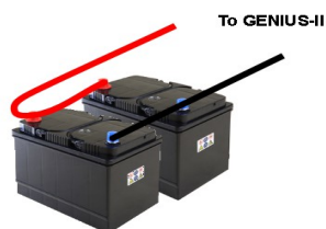
Figure 4: Recommended wiring for connecting batteries in parallel
